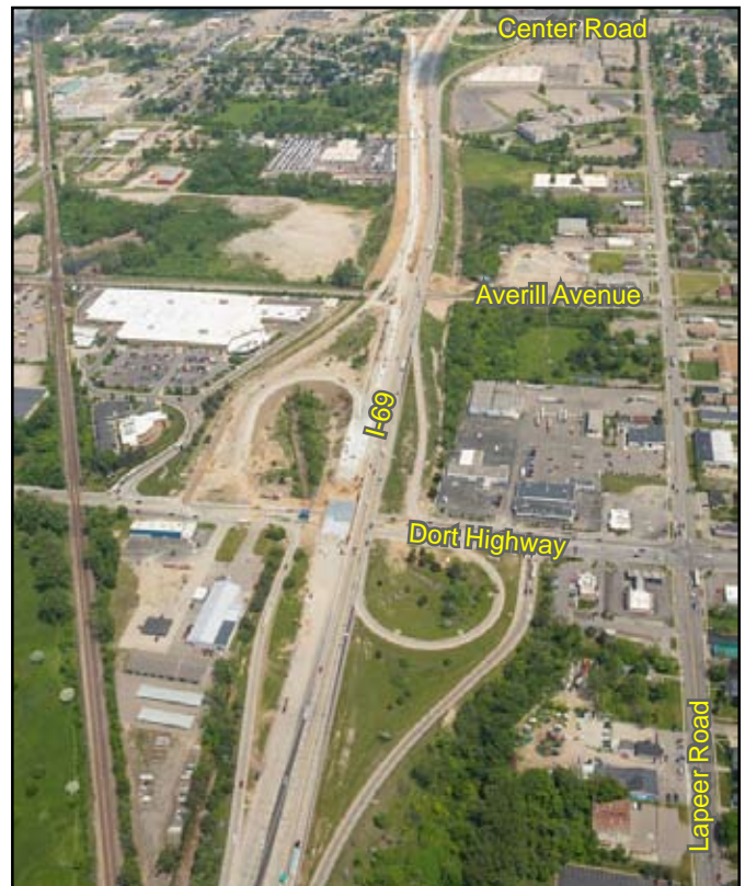
Above is I-69 over Averill Avenue. Existing bridges were widened with micropile-supported foundations. At right is the Dort Highway (M-54) interchange. Complete reconstruction of both overpass structures will allow additional height for vehicles traveling on Dort Highway.
